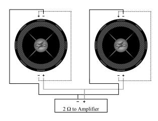
Wiring method of two MOFO's to a monoblock amplifier with a **2 ohm RMS** rating the same as both MOFO's **RMS** ratings added together.
