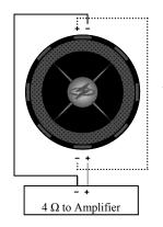
Wiring method of 1 MOFO to a 2 channel amplifier with a 4 ohm bridged RMS rating the same as the MOFO's RMS rating.
